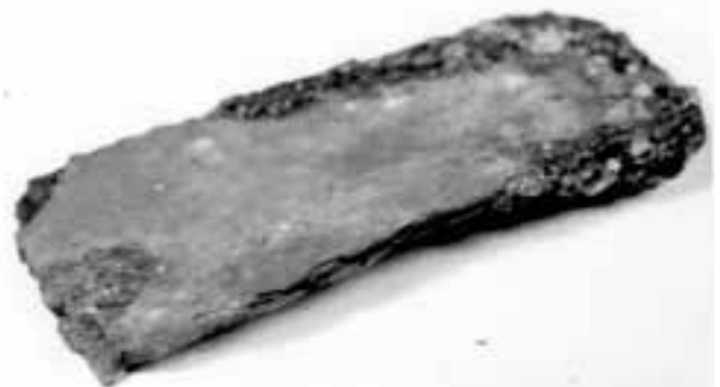
Figure 17: A decarburised iron plate excavated from the Guxing ironworks site in Zhengzhou, Henan Province.
