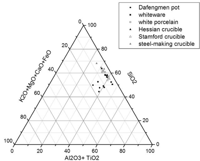
**Fig. 8.** Ternary diagram of SiO<sub>2</sub>–(Al<sub>2</sub>O<sub>3</sub> + TiO<sub>2</sub>)–(K<sub>2</sub>O + MgO + CaO + FeO) showing the matrix compositions of the Dafengmen pots and some kaolinitic ceramics: Neolithic and Shang whitewares (Kerr and Wood, 2004), Ding white porcelains (Kerr and Wood, 2004), Hessian crucibles (Martinón-Torres and Rehren, 2009), Stamford crucibles (Freestone and Tite, 1986) and Central Asian steel-making crucibles (Rehren and Papachristou, 2003).
