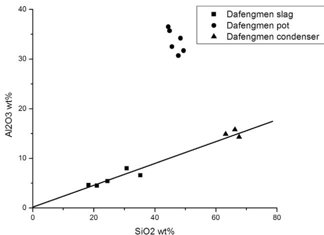
Fig. 10. The SiO<sub>2</sub> and Al<sub>2</sub>O<sub>3</sub> contents in the slag, pot and condenser samples from Dafengmen. Note the linear correlation of the SiO<sub>2</sub> and Al<sub>2</sub>O<sub>3</sub> contents of the slag and condenser samples.
