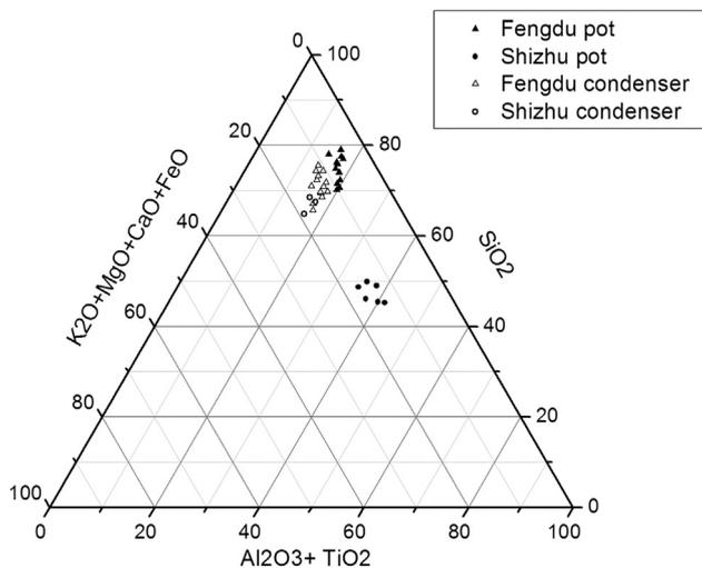
**Fig. 7.** Ternary diagram of SiO<sub>2</sub>–(Al<sub>2</sub>O<sub>3</sub> + TiO<sub>2</sub>)–(K<sub>2</sub>O + MgO + CaO + FeO) showing the bulk compositions of the pot and condenser fabrics from Fengdu (three sites) and Shizhu (Dafengmen).
