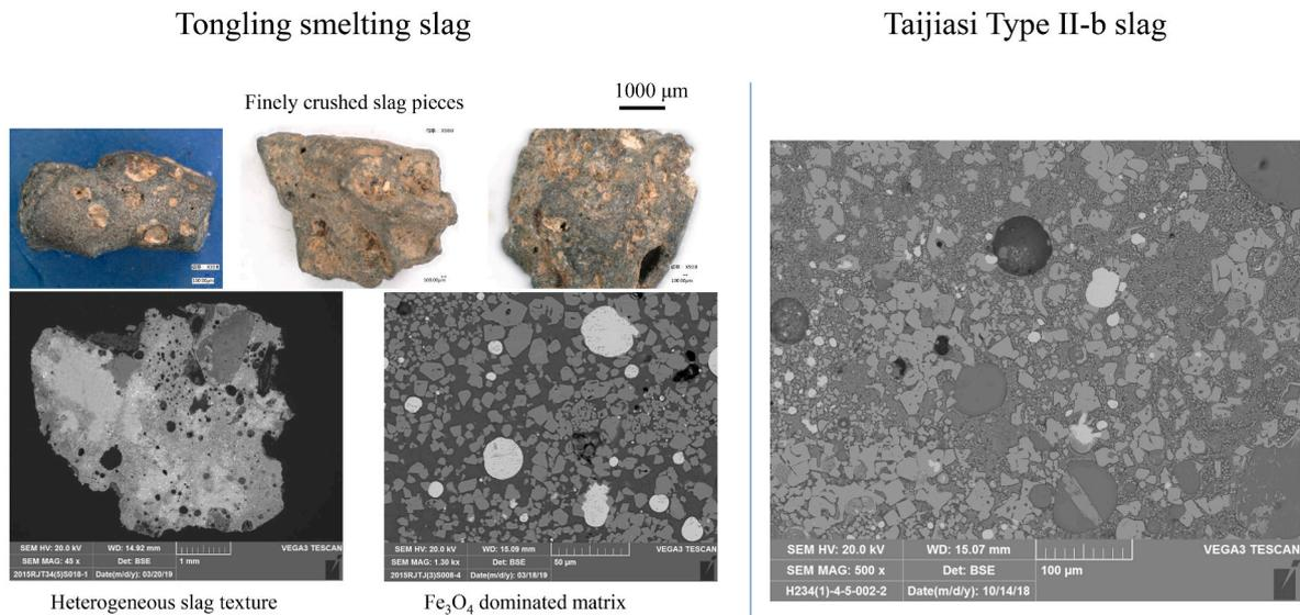
Fig. 12. The comparison between Tongling and Taijiyasi Type II-b slag. Their mineralogical compositions and heterogeneity are quite similar to each other.
