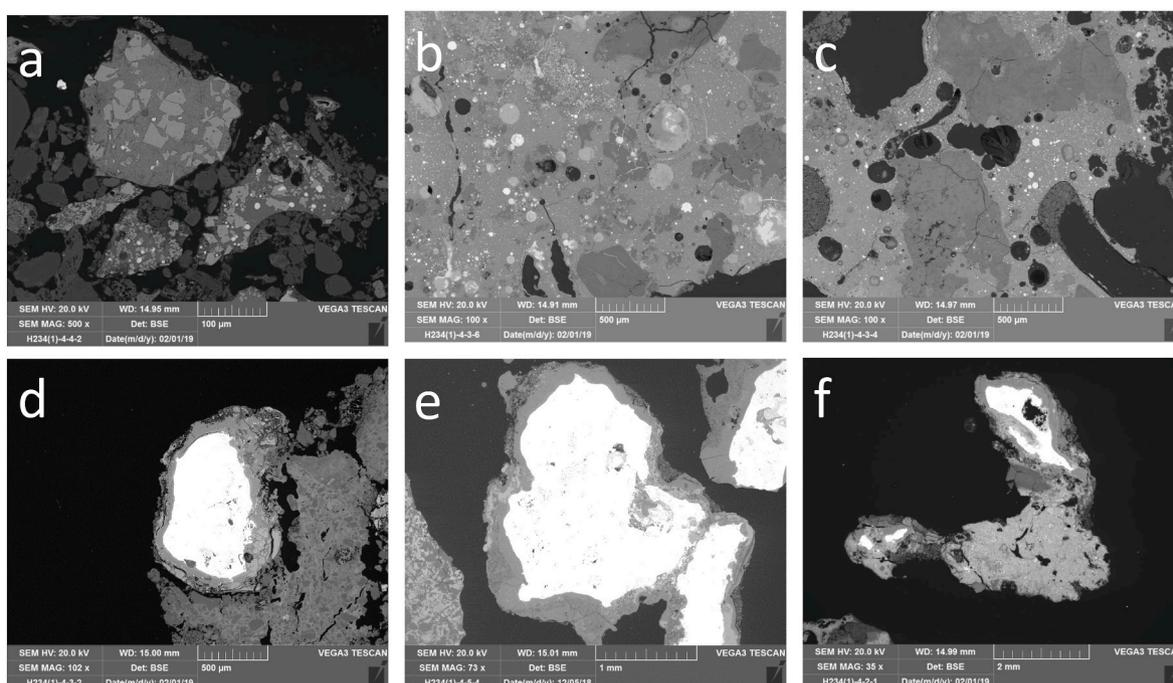
**Fig. 9.** Micrographs of Type II slag. a: slag fragments with angular magnetite crystals. b, c: relatively large slag fragments containing unreacted quartz particles. d, e, f: metallic prills embedded in Type II slag.
