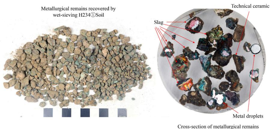
**Fig. 5.** Micro-artefacts recovered from the H234① soil samples. The diameter of the resin block is 3 cm. Many of the fragments in the left picture are conglomerates of many slag pieces, bound by clay matrix. The actual particle size of slag can only be measured by microscopic analysis.
