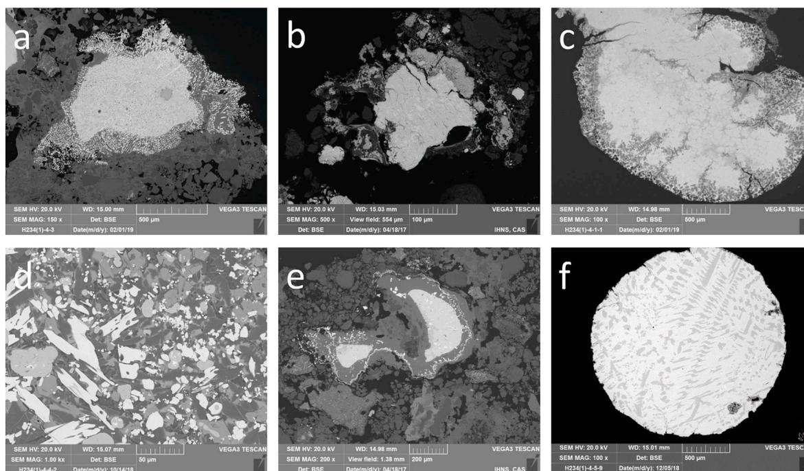
Fig. 7. Micrographs of Type I slag, dross and metal prills. a,e: Typical burnt metal with a large metal core surrounded by tin oxides. d: matrix of Type I slag with many tin oxide and copper oxide crystals. b,c,f: Metallic prills/fragments with varied tin content.
