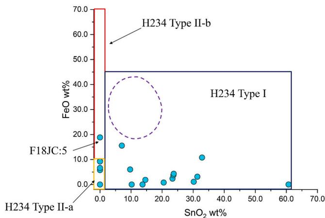
**Fig. 11.** Chemical composition of slag samples from other contexts. The compositional range of H234 Type I and Type II slags are indicated with blue and red/yellow rectangles, respectively. (For interpretation of the references to colour in this figure legend, the reader is referred to the Web version of this article.)
