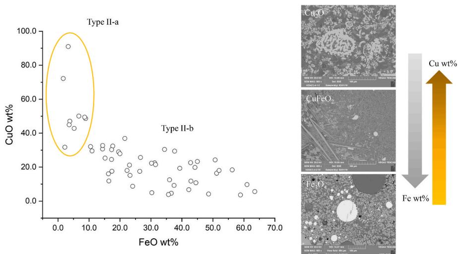
**Fig. 8.** Chemical and mineralogical composition of Type II slag samples. Their typical microstructure changes along with Fe and Cu content. Type II-a slag are rich in Cu but poor in Fe. Type II-b slag are rich in Fe.
